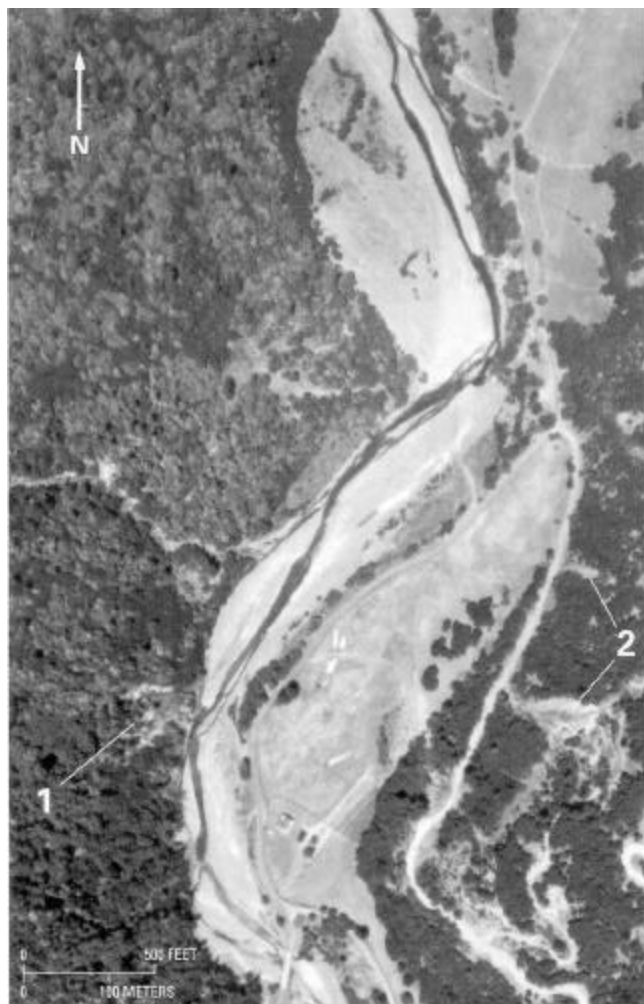
FIGURE 6.—Protective influence of flood plains on streamside hillslopes. Streamside landslides are numerous where Redwood Creek abuts hillslopes directly (1). On opposite bank, landslides (2) are separated from the active channel by a low flood plain. The photograph depicts the main channel of Redwood Creek immediately below the mouth of Minor Creek.
