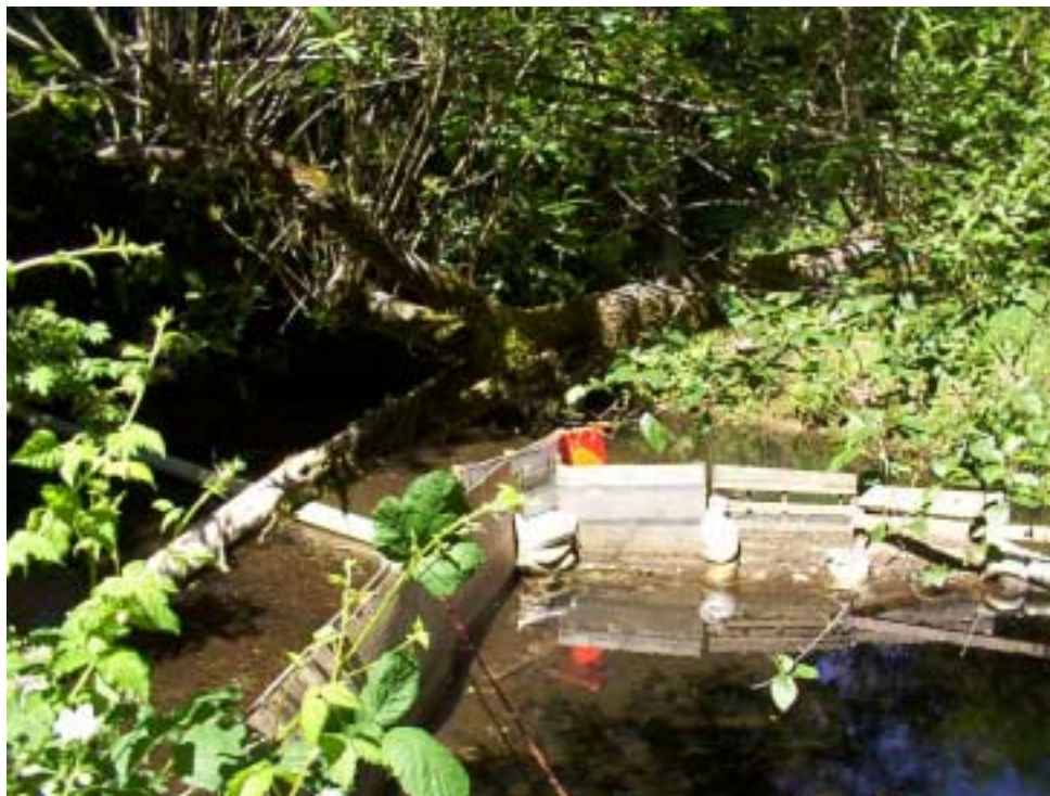
Figure 1. Full channel weir funneling water and fish into PVC pipe.
