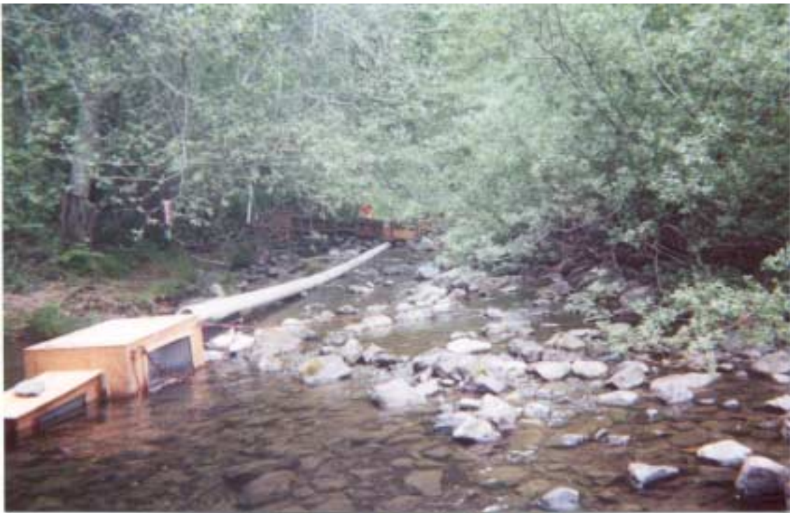
Figure 1. Full channel weir funneling water and fish into PVC pipe.
