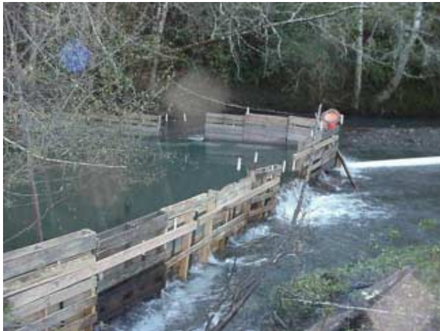
Figure 1. Weir funneling water and fish into PVC pipe.
